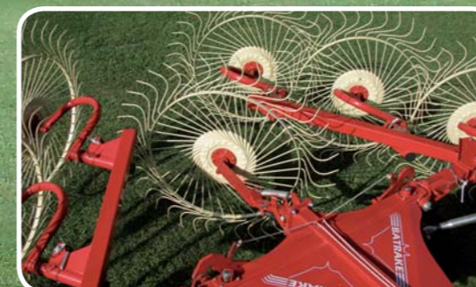
Optional hydraulically raised Kicker wheel available for all sizes
